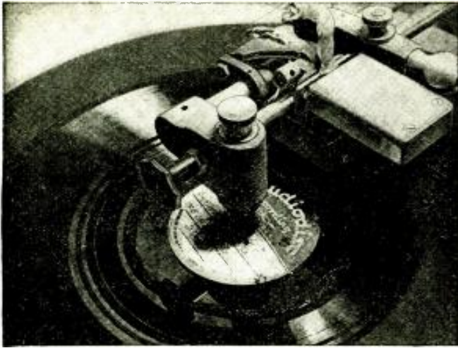
Recorder working well, chip thrown clear and moving toward center.
