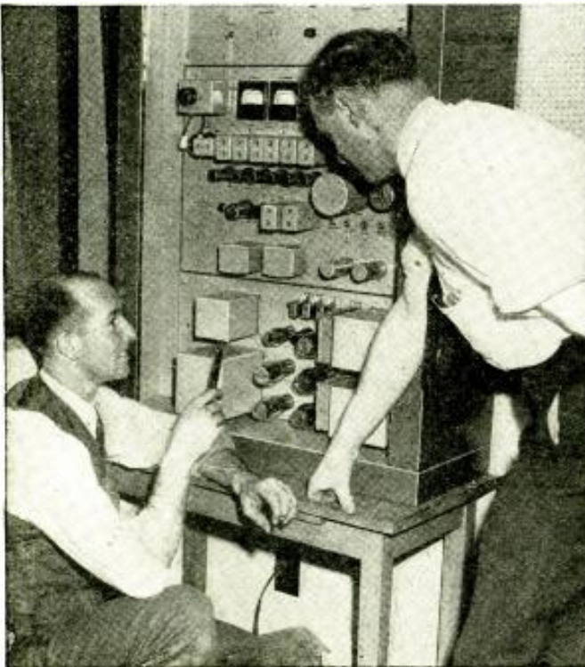
The 2½-watt transmitter used to broadcast to the student body of Syracuse University.
